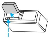
3. Turn the magazine (A) over.4. Using the disc holder release knob (C), pull the disc holder (B) out of the magazine.
